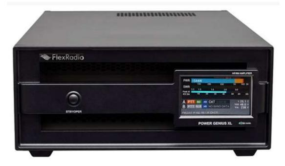
The PowerGenius XL is a 100% duty cycle, legal limit (1500W ICAS) 1.8-54 MHz RF amplifier intended for both amateur and government use. It incorporates a pair of modern NXP MRF1K50H LDMOS transistors that are individually capable of 1.5 kW thus providing plenty of headroom for lowest IMD and spurious output. Efficiency and spurious performance are also enhanced through the use of diplexed filters.
