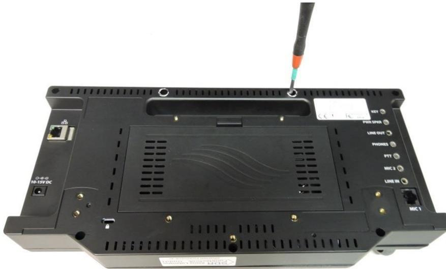
Using the #2 Phillips screwdriver, reinstall the tilt feet or the fixed tilt stand on the Maestro.
