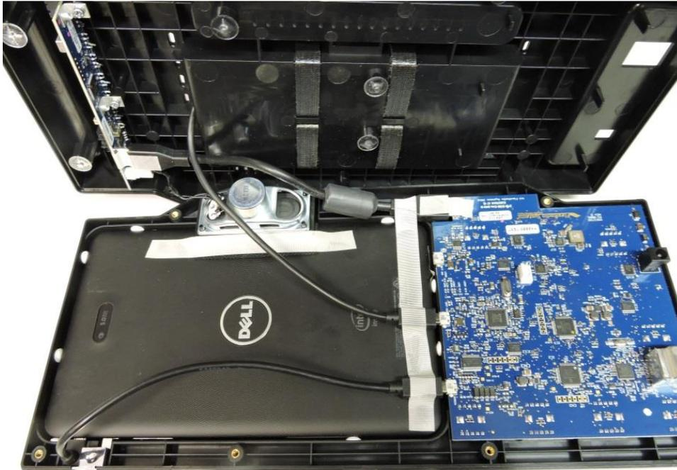
Properly orientate the thick audio cable with the ferrite core around the bottom of the speaker as shown below.
